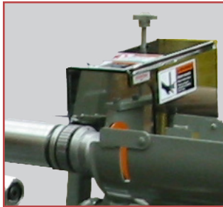
Double guarded fixed knife for operator safety
