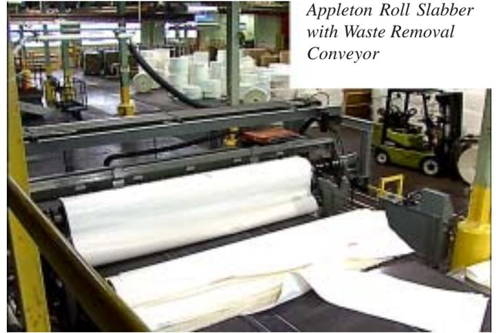
*Appleton Roll Slabber with Waste Removal Conveyor*
