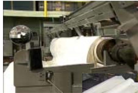
*Steel Wedges Peel Waste Paper From Reel*
