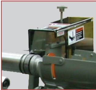
Double guarded fixed knife for operator safety
