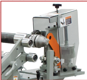
Double Guarded Fixed Knife for Operator Safety
